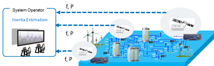
Figure 1: Inertia Estimation Concept for Monitoring Purposes
